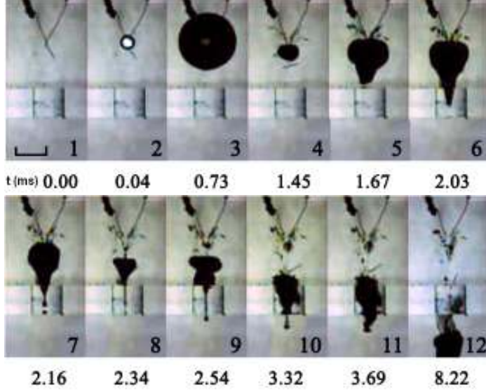
Figure 3. A collapsing bubble in a fluid of viscosity \mu = 900 mPas at a non-dimensional distance H' = 1.5 . The maximum radius of the bubble is R_m = 4.9 mm (Frame 3). The jet from the bubble enters the hole in Frame 5. Note the break-up of the jet from the main bubble in Frame 7 as the main bubble shrinks in its oscillation cycle. The scale bar shown in Frame 1 corresponds to 5 mm.
